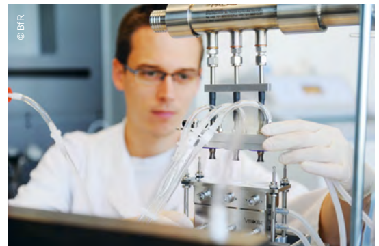
Test setup: three tubes conduct a test aerosol with airborne nanomaterials to epithelial cells.
