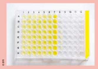
Double dose: microtiter plates allow for the parallel testing of chemicals in varying concentrations.
