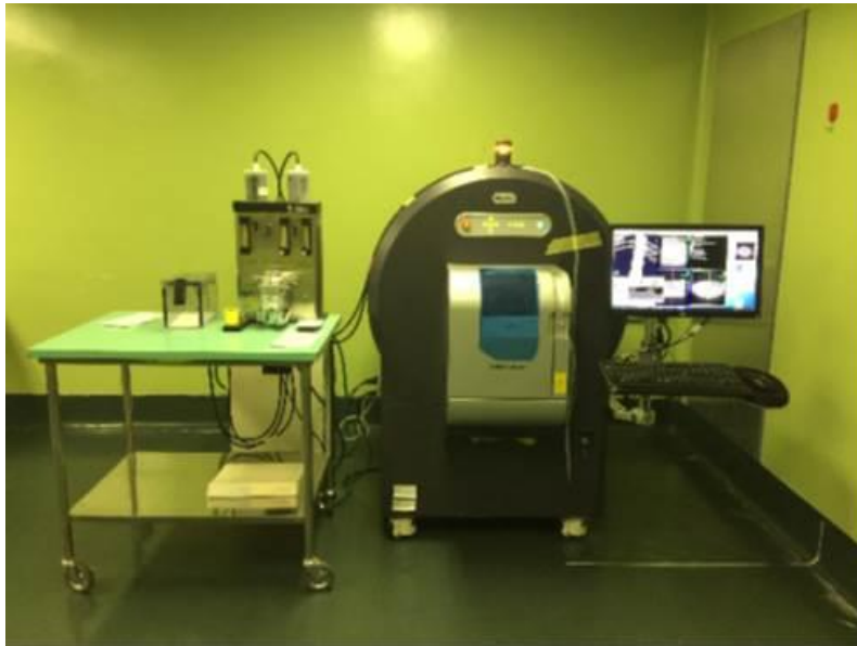
3D micro X-ray computed tomography (CT) for laboratory animals CosmoScan GXII (RIGAKU, Japan)
