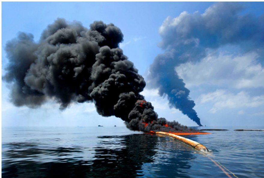
Figure 10: Controlled in situ burning in the Gulf of Mexico after contain- ing the oil with a fire boom (Picture source: U.S. Navy, MCS Justin Stumberg).
